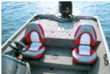
■ *Lowe's 180W Stinger was a decent performer with its Mercury 150 OptiMax, but it was rigged conservatively, which hurt top-end speed and handling. Holeshoot was the best of the bunch at 4.6 seconds. The dash didn't flex at all despite an abundance of plastic fascia. Folding seats provided good support in rough water.*
