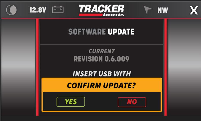
The system will reboot to a status bar and animation on the touch display. This status bar shows the user the progress of the software update. Once the software update is complete, the system will reboot into the application. You may then remove the USB drive.
