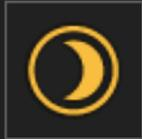
The Night Mode button toggles the back-lighting between the daytime and nighttime set points. This can be adjusted in the System Display section of the Settings menu.
