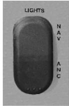
Three-position (Nav/Anc/Off) switch that activates the navigation running lights (when installed) for night operation. NAV position - turns on the red and green bow lights and white stern light as well as illuminates instrument lights. ANCHOR position - turns on stern light only for night anchoring. Do not operate the boat with the switch in the ANCHOR position only.
