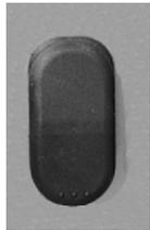
Three position switch that activates the livewell pump to either fill or recirculate water from the livewell tank. Make sure the switch is turned off when not in use to avoid damaging the pump.
