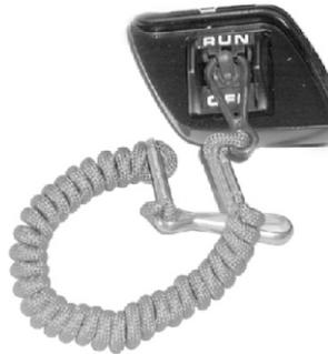
slide the black plastic loop over the toggle switch and flip the switch.
