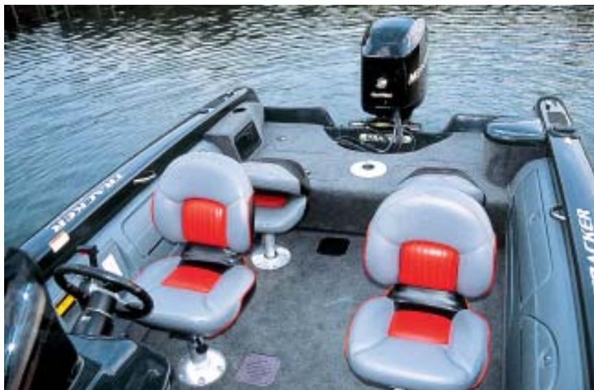
■ The 18 SC features four swiveling, sliding and locking pedestal seats. The driver and helm seats employ a shock-absorbing suspension system to soften the ride in rough water.
