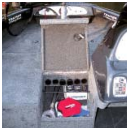
■ Beneath the front deck is a dual-level centerline rod locker with organizer tubes flanked by separate lockable storage compartments port and starboard.
